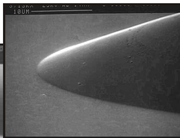
The SEM shows a lens etch stopped at 90 % of the total etch time.
