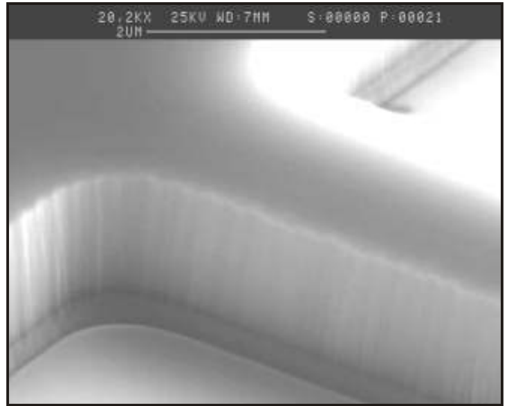
AlGaIn/ GaN etch GaN etch rate > 0.6 µm/min Sel to Oxide >7:1 Anisotropic profile Smooth sidewalls Clean etch surface
