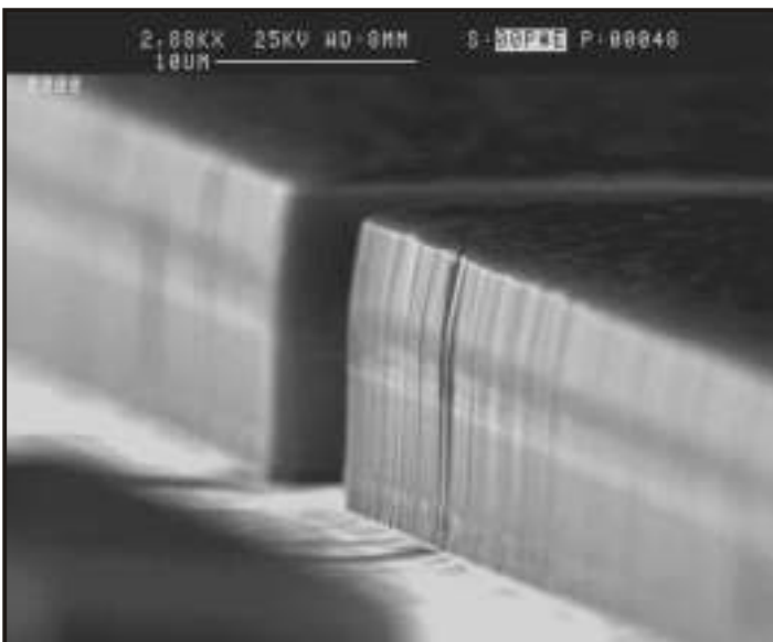
GaP/InGaAlP etch rate > 0.6µm/ min selectivity to SiO 2 > 8 : 1
