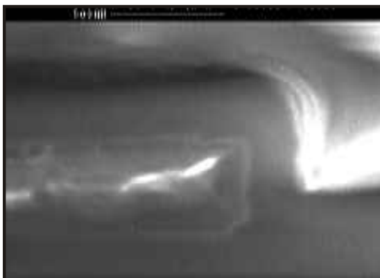
0.3 µm SiO 2 deposited over a 0.5 µm step
