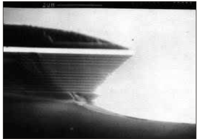
ca. 5 \mu\text{m} deep etch under different angles (without substrate rotation) Photoresist Mask intact (not removed)
