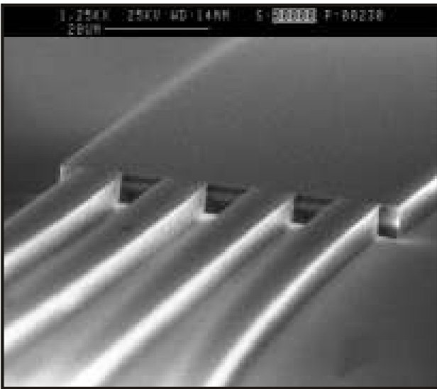
OPT application lab, Yatton/ UK: top left: 8 μm deep, anisotropic SiO 2 ICP-RIE
