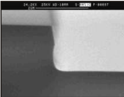
1,6 \mu\text{m} deep, anisotropic etch (SiO 2 mask still in place)
